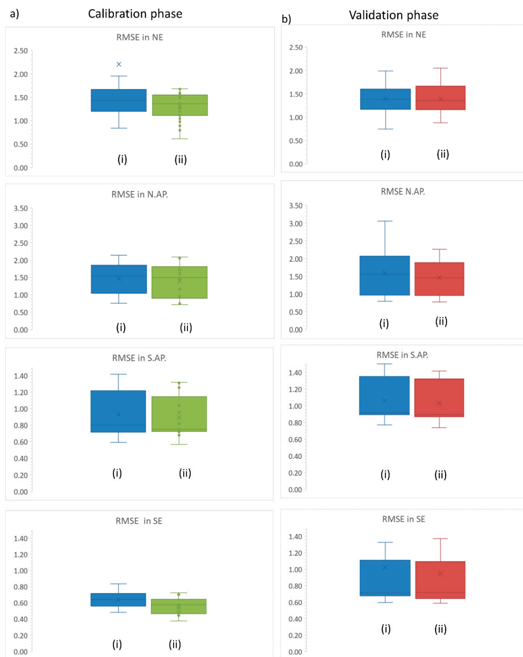
Figure 5. RMSE results calculated from predicted and simulated discharges using a priori and calibrated parameters in calibration (panel (a) of the Figure) and validation (panel (b) of the Figure). In panels (a,b), the boxplots (i) used the a priori parameters and the boxplot (ii) used the calibrated parameters. NE stands for north east, N.AP. stands for North Appalachian, S.AP. stands for south Appalachian, SE stands for south east.
